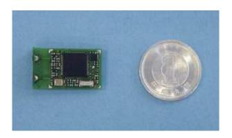
Panasonic, the leading brand by which Matsushita Electric Industrial Co., Ltd. is known, today unveiled its ultra-small low-power wireless module by incorporating a radio circuit and a microcomputer onto a single CMOS LSI chip, the world's first in 400-MHz band low-power wireless technology. The tiny high-speed wireless module is suitable for a wide range of home and industrial applications.
