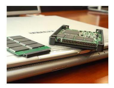
Samsung Electronics today announced that it has developed the first Solid State Disk (SSD) based on NAND Flash memory technology. The NAND-based SSD is a low power, lightweight storage media for notebook PCs, sub-notebook PCs and tablet PCs. Using the industry's highest density 8Gb NAND Flash, Samsung can build SSDs with a capacity of up to 16Gb.
