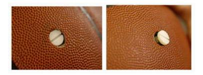
A tiny, battery-powered sounding device is placed inside this Spalding Infusion basketball in a cavity usually used for an air pump. Photo by Will Kirk
