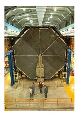
A new physics experiment combines thousands of tons of steel plates, a powerful particle accelerator and 450 miles of solid rock to reveal the secrets of a particle that sometimes seems to barely exist. Researchers in Argonne's High Energy Physics Division were instrumental in getting the experiment, called the Main Injector Neutrino Oscillation Search (MINOS), launched in the late 1980s, and later
