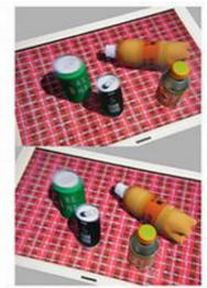
Flatbet 3-D Display (Above) Display viewed from left (Below) Display viewed from right The can with the orange and yellow cap, on the bottom right, is real; the other objects are generated by the display
