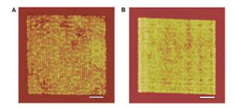
At left (A) is an image of an array of nanowires 60 nanometers wide created with the silver superlens. The center distance between each nanowire is 120 nanometers. To the right (B) is an image of the same nanowires. In this image, created without the superlens, the individual nanowires are not distinct. The scale bar on both images is 1 micrometer.
