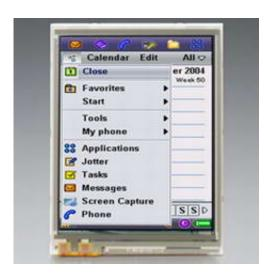
NEC LCD Technologies, Ltd. today announced that sample shipments of its 2.7-inch (6.8cm diagonal), quarter video graphic array ("QVGA"), amorphous silicon thin-film-transistor liquid crystal display ("TFT LCDs"), part number "NL2432HC17-01B," will commence in June 2005. This model realizes high contrast, vivid display, and low power consumption making it ideal for use in mobile terminals.
