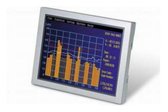
NEC LCD Technologies, Ltd. today announced that sample shipments of its new 5.5-inch (14cm-diagonal), quarter video graphics array (QVGA), amorphous silicon, thin film transistor liquid crystal display (TFT LCD) module, part number NL3224BC35-22, will commence in June 2005. This is the first module introduced by NEC LCD Technologies that features its newly developed Super-Transmissive Natural Light TFT ("ST-NLT") technology. This new technology delivers vivid colors even in direct sunlight.
