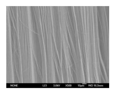
First Nano grows high-density vertically aligned carbon nanotubes over 1 mm long.
