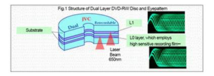
Newly Developed High Sensitive Recording Film and a New Writing Method "N-Strategy" to Enhance Erasability Produce Dual Layer DVD-RW Disc 8.5GB Disc for Up to 11 Hours of Video Recording
