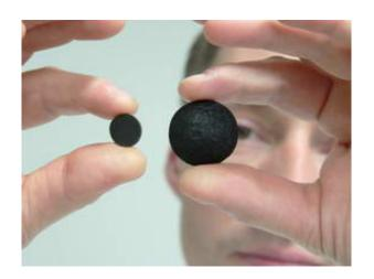
Cracks, splits and holes are by definition one of the biggest problems in sealing technology. A new addition has recently been made to the thermoplastic elastomer family: Swellable variants of these plastics react to leaking water and thus stop the leaks.
