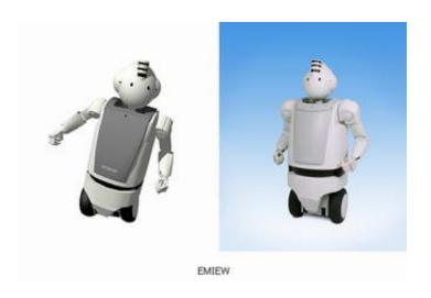
Hitachi, Ltd. announced that it has developed a robot - called "EMIEW"\* - for supporting people's everyday lives. EMIEW has the physical capabilities, such as agile movement and obstacle avoidance, needed for real life, and can move around while interacting in dialog with humans from a distance of one meter without the need for microphones. The technologies developed for EMIEW will lead the way in creating robots of the future that can cooperate and coexist with humans.
