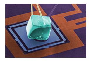
Chip-scale refrigerators capable of reaching temperatures as low as 100 milliKelvin have been used to cool bulk objects for the first time, researchers at the National Institute of Standards and Technology (NIST) report. The solid-state refrigerators have applications such as cooling cryogenic sensors in highly sensitive instruments for semiconductor defect analysis and astronomical research.
