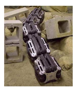
A virtually unstoppable "snakebot" developed by a University of Michigan team that resembles a high-tech slinky as it climbs pipes and stairs, rolls over rough terrain and spans wide gaps to reach the other side.
