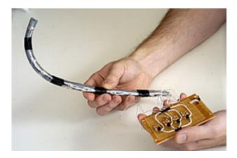
Can a robot learn to navigate like a cockroach? To help researchers find out if a mechanical device can mimic the pesky insect's behavior, a Johns Hopkins engineering student has built a flexible, sensor-laden antenna. Like a cockroach's own wriggly appendage, the artificial antenna sends signals to a wheeled robot's electronic brain, enabling the machine to scurry along walls, turn corners and avoid obstacles.
