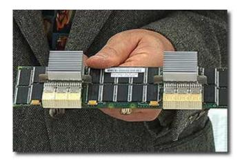
Image above: The unique BlueGene/L "compute card" consists of two nodes, each containing two central processing units (CPUs) including four megabytes of dedicated memory. Also mounted on the circuit board are a memory controller module and nine separate memory chips, similar to those in standard home and office desktop computers.
