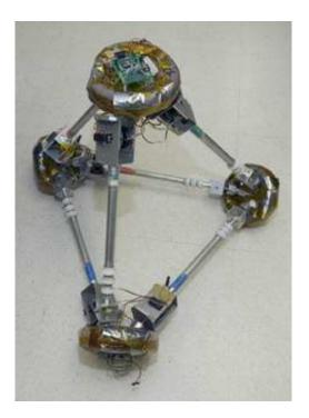
Like new and protective parents, engineers watched as the TETWalker robot successfully traveled across the floor at NASA's Goddard Space Flight Center in Greenbelt, Maryland. Robots of this type will eventually be miniaturized and joined together to form "autonomous nanotechnology swarms" (ANTS) that alter their shape to flow over rocky terrain or to create useful structures like communications antennae and solar sails. This technology has the potential to directly support
