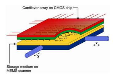
Image: The "millipede" concept: For operation of the device, the cantilever tips are brought into contact with the storage medium — a thin film of a specific cross-linked polymer coated on a silicon substrate, which is moved in the x- and y-directions for reading, writing, and erasing. The storage medium is positioned with nanometer-scale accuracy relative to the cantilever array. The tips can independently read, write or erase the bits.
