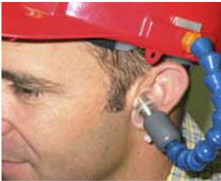
The device uses infra-red rays to measure changes in ear temperature, which the researchers say indicates which 'side' of the brain is more active.
