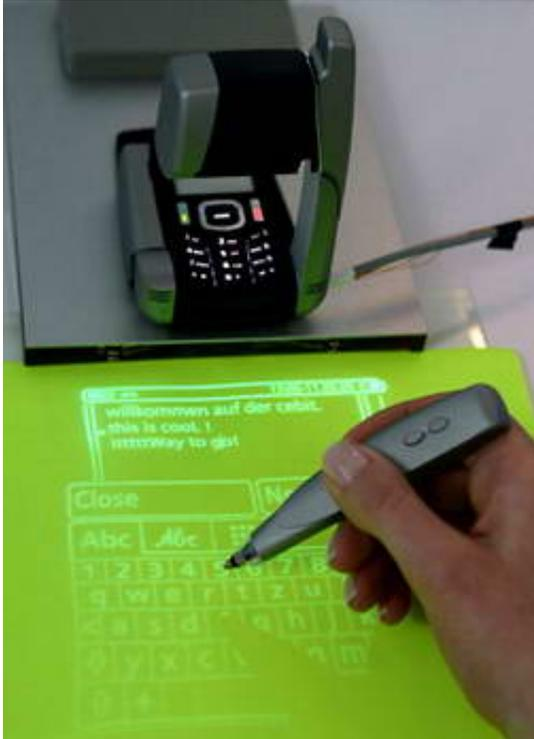
Siemens researchers have developed a cell phone featuring a built-in projector system. A laboratory model was presented at CeBIT 2005 in Hanover. The system makes it possible to project a complete keypad or display onto a surface. With a special pen, users can write on the virtual keypad and operate the phone's functions.
