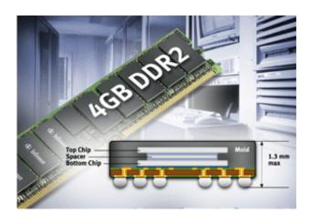
Infineon Technologies AG, demonstrating its leadership as memory supplier, announced that it is sampling the industry's first dual-die based 4GB (Gigabyte) DDR2 registered DIMMs (Dual Inline Memory Modules) for server applications. The new module is based on eighteen 2Gbit (Gigabit) DDR2 components, realized by stacking two 1Gbit DDR2 SDRAMs. This approach called Dual Die technology allows to double memory density while increasing component height by only 0.1mm.
