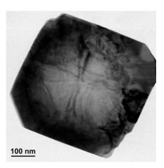
Using high-intensity ultrasound, researchers at the University of Illinois at Urbana-Champaign have created hollow nanospheres and the first hollow nanocrystals. The nanospheres could be used in microelectronics, drug delivery and as catalysts for making environmentally friendly fuels.
