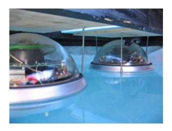
Working under harsh Antarctic conditions, an international team of scientists, engineers and technicians has set in place the first critical elements of a massive neutrino telescope at the South Pole. The successful deployment - in a 1.5 mile-deep hole drilled into the Antarctic ice - of a string of 60 optical detectors designed to sample phantom-like high-energy particles from deep space represents a key first step in the construction of the \$272 million telescope known as IceCube.
