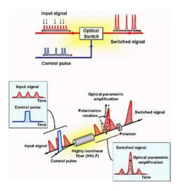
Figure: Functions of new optical switch (upper diagram) and conceptualized diagram of switching principle (lower diagram: input signal is amplified timed with control pulse, as shown in the insets)
