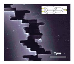
Under stress, tiles of calcium carbonate can slide, absorbing energy. Because of this microstructure, the abalone shell can absorb a great deal of energy without failing.
