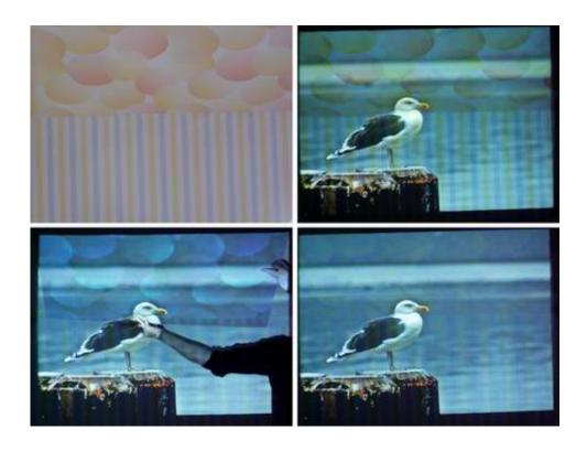
Image: Projection onto a pitched roof area. The image sequence shows (a) the wallpapered surface, (b) the projection with uncorrected colors, (c) color correction projected onto a white piece of paper, and (d) the color-corrected image on wallpaper. All projections are geometry corrected.
