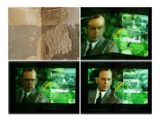
Image: Projecting images onto environmental surfaces. (a) A scruffy corner serves as the projection surface. (b) The uncorrected image. (c) The projector system corrects the image's geometry and, finally, (d) its color. Displayed content: The Jackal, Universal Pictures.
