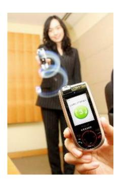
Samsung Electronics unveiled the world's first "3D movement recognition" mobile phone SCH-S310. 'Accelerometer' is built in to accurately calculate and ascertain movement in three dimensional space and then carry out commands according to those calculations. Sophisticated sensing technology calculates the direction in which the mobile phone is moving as well as its speed of movement. The capability
