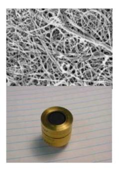
Carbon nanotubes (top) are applied to a NIST-developed pyroelectric detector (bottom) that may improve thermal conductivity and resistance to laser damage. Credit: NIST
