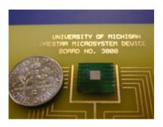
University of Michigan researchers are developing ways that could produce fuel cells at a fraction of the current cost by using microfabrication rather than traditional manufacturing processes. "We arrived at a system that works and uses steps that are very similar to those used to make microelectronic devices," said Levi Thompson, U-M chemical engineering professor and leader of the research team working on the technology.
