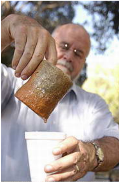
Tony Flynn demonstrates the simple water filter, which removes over 95 per cent of pathogens.
