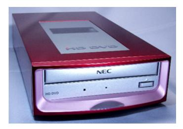
NEC Corporation today announced that it has completed the development of technology capable of playing back HD DVDs, DVDs, and CDs with a single optical head, enabling creation of the world's first half height size drive suitable for desktop computer installation.
