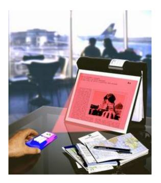
The vest-pocket projector could soon become reality. It is based on a tilting micromirror that builds up the picture line by line. The designers of a laboratory prototype have managed to raise its operating speed and resolution to the point where graphics and text are clearly legible.
