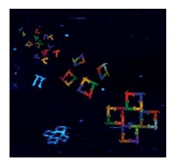
AFM image of a cross-shaped jigsaw puzzle of 4 tectosquares - 3D models depict process of assembly.
