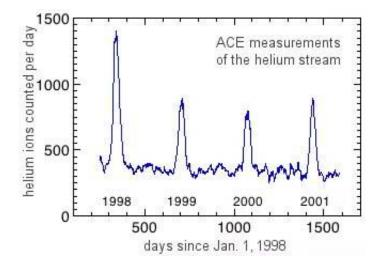
Image: ACE/SWICS measurements of the helium stream. Peaks denote annual passages through the focusing cone. Click on the image to see the complete 7-year data set.
