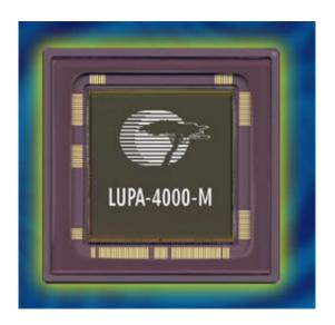
Cypress Semiconductor Corp today announced commercial sampling of the LUPA-4000-M CMOS image sensor from recently acquired FillFactory NV. Developed to address the specific imaging needs of the professional and industrial market place, the LUPA-4000-M's target applications include machine vision, instrumentation, surveillance, biometric identification and medical imaging.
