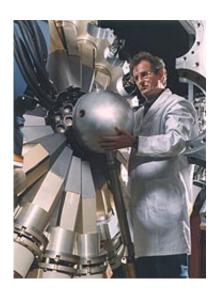
**Gammasphere**, the world's most sensitive gamma-ray detector, is already a seasoned traveler, having crossed the United States from Lawrence Berkeley National Laboratory to Argonne by truck, but the 20-ton instrument has recently gone truly mobile and can now be moved around the experiment hall in Argonne-East's Building 203 to meet the needs of physicists.
