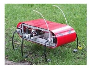
A cockroach-like <u>robot</u> named RHex is the starting point for a major project to **understand animals' most distinguishing trait - how they move without falling over**.
