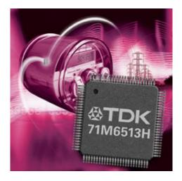
TDK Semiconductor Corp., a leader in the design and manufacture of mixed-signal semiconductors for world markets, today unveiled the world's first true system-on-chip for industrial poly-phase power meters. The new TDK 71M6513H integrates a 21 bit delta-sigma-delta converter, 32-bit compute engine, MCU, RTC, LCD driver, and ultra-precision voltage reference and provides better than 0.1% accuracy with only a few low cost external components.
