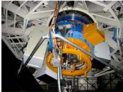
SINFONI Adaptive Optics Module at VLT Yepun (June 2004) ESO PR Photo 24/04 (24 August 2004) © European Southern Observatory
