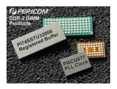
Pericom Semiconductor Corporation (NASDAQ:PSEM), a worldwide preferred supplier of high-speed integrated circuits and frequency control devices, today announced the release of its industry leading performance DDR2 Registered Buffers and PLL Clock for Registered <u>DIMMs</u>. These DIMMs are found in next generation higher performance systems such as servers, routers, switches, and workstations.
