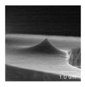
Microcantilever heaters fabricated by the research group of William King at Georgia Tech. The microcantilevers are made of crystalline silicon, and have been engineered with atomic impurities that allow electricity to flow through them. The cantilevers he
