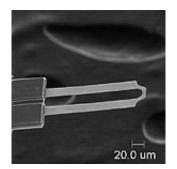
Combining thousands of individually-controlled AFM pens into arrays could allow writing of complex semiconductor patterns. King says the thermal dip pen technique could produce features as small as ten nanometers, well beyond the limits of conventional semiconductor patterning processes that depend on light projected through a lithographic mask.
