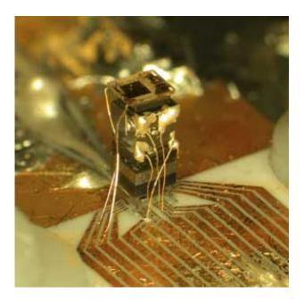
The heart of a minuscule atomic clock---believed to be 100 times smaller than any other <u>atomic clock</u>---has been demonstrated by scientists at the Commerce Department's National Institute of Standards and Technology (<u>NIST</u>), opening the door to atomically precise timekeeping in portable, battery-powered devices for secure <u>wireless</u> communications, more precise navigation and other applications.
