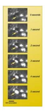
A <u>nanocrystalline metal</u> is one whose average grain size is measured in billionths of a meter, much smaller than in most ordinary metals. As the grain size of a metal shrinks, it can become many times stronger, but it also usually loses ductility. To take advantage of increasing strength with decreasing grain size, researchers must first understand a fundamental problem: **by what processes do nanosized crystals of metal stretch, bend, or otherwise deform under strain?**
