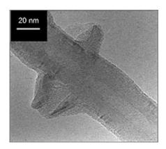
Diamonds are the hardest known substance. Carbon nanotubes are the strongest. Scientists at the U.S. Department of Energy's Argonne National Laboratory tried to **combine the best of both worlds by creating a composite nanostructure**. They wanted to grow tiny carbon tubes with tiny diamonds.
