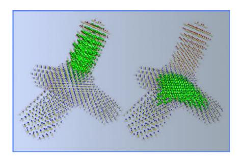
NERSC calculations using local density approximation, the charge patching method, and the folded spectrum method yield atom-by-atom electronic maps of a tetrapod with one leg of cadmium selenide and three of cadmium telluride.
