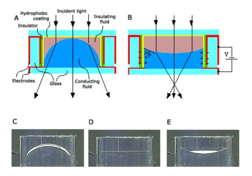
(A) Schematic cross section of the FluidFocus lens principle. (B) When a voltage is applied, charges accumulate in the glass wall electrode and opposite charges collect near the solid/liquid interface in the conducting liquid. The resulting electrostatic force lowers the solid/liquid interfacial tension and with that the contact angle  $\theta$  and hence the focal distance of the lens. (C) to (E) Shapes of a 6-mm diameter lens taken at different applied voltages.
