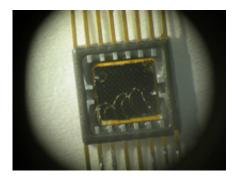
Researchers at the University of Southern California and the University of Texas at Austin have built and tested a device based on nanostructures called quantum dots that can sensitively detect infrared radiation in a crucial wavelength range. Quantum dot IR receptor unit.
