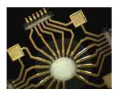
There is a continuous drive towards further integration and miniaturization in electronic modules and components. This generates a constant need for new or improved manufacturing technologies for IC's and IC based modules. Philips CFT (Centre for Industrial Technology) has developed an **ingenious 3-dimensional interconnection pattern technology based on photolithography using inclined UV exposure, resulting in relatively lower costs, miniaturization and more design freedom**.
