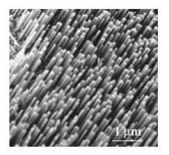
Xuan Wang et al. from Peking University, China report in the last issue of Applied Physics Letters about ZnO nanowires grown through evaporation of zinc powders under a low temperature of 400 C. Being about 10 nm in the diameter these nanowires are long and curved. Typical lengths are tens of micrometers. High-resolution transmission electron microscopy showed that nanowires are mostly crystalline.
