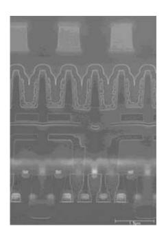
Renesas Technology Corp. has developed the industry's first SRAM virtually free of soft errors, dubbed "superSRAM", through the development a new type of memory cell combining an SRAM cell with a DRAM capacitor technology. This new SRAM will be applied to, and put into commercial production for, the 16M-bit low-power SRAM for mobile applications. Details will be announced at the 2004 Symposium on VLSI Technology to be held in Hawaii in the United States on June
